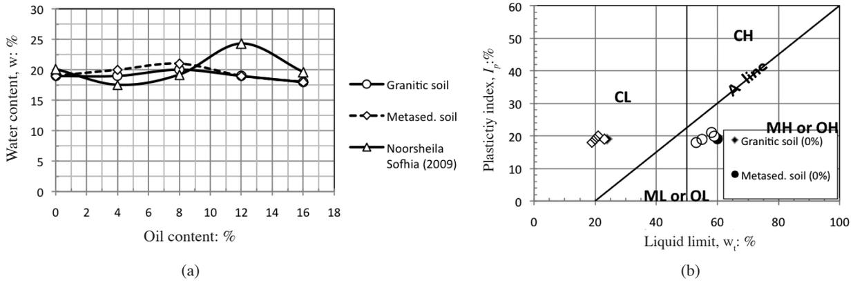
FIGURE 4. (a) The trends of plasticity index ( $w$  %) and (b) data points on the plasticity chart, taken from Unified Soil Classification System. CH: inorganic clays of high plasticity; CL: inorganic clays of low to medium plasticity
