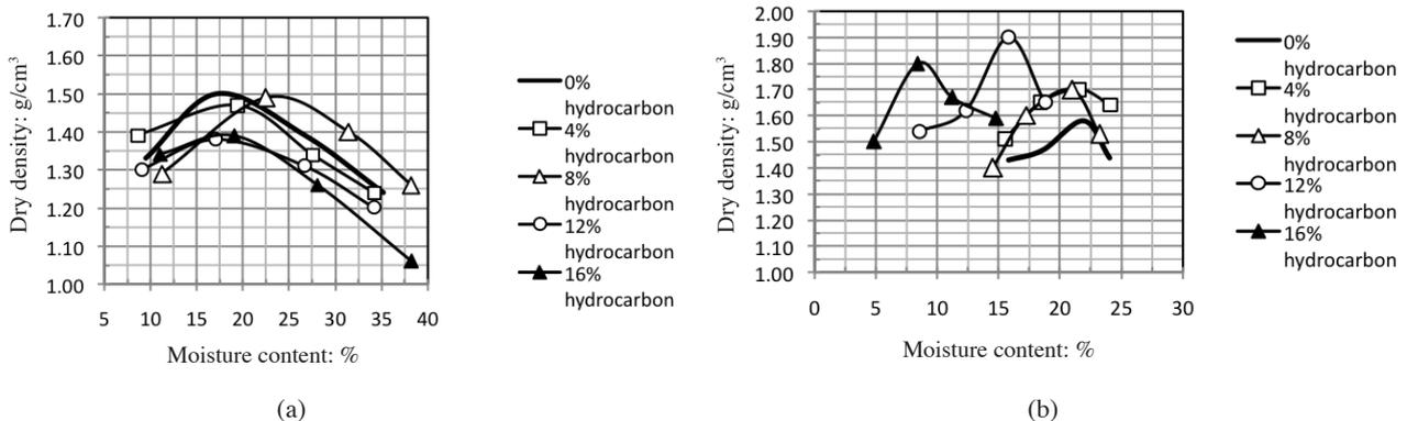
FIGURE 5. Compaction curve for (a) granite soil and (b) for metasedimentary soil
