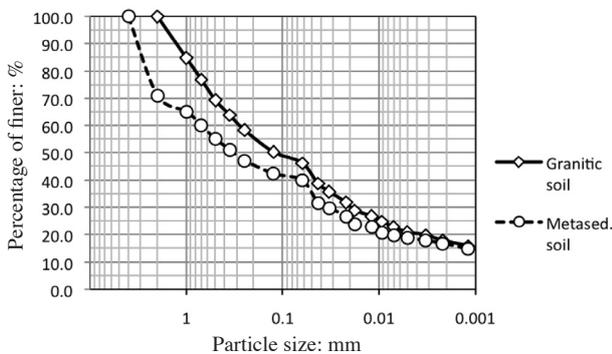
FIGURE 2. The particle size distribution curves of both types of soils
