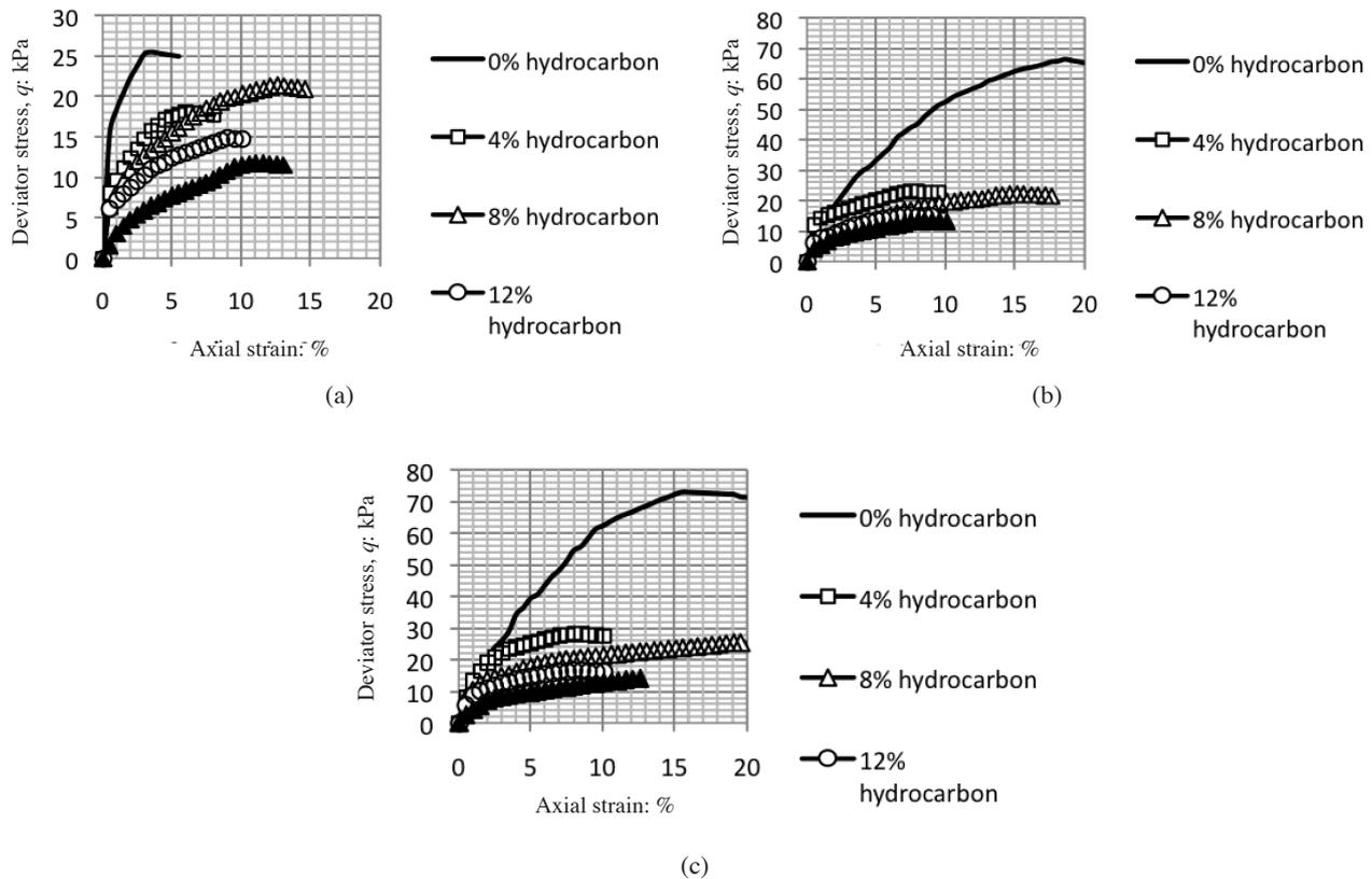
FIGURE 8. The relationship between deviatoric stress and strain for granite soil with different applied confining pressures of (a) 140 kPa, (b) 280 kPa, and (c) 420 kPa
