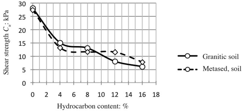
FIGURE 6. Shear strength values,  $C_u$  for granitic and metasedimentary soils
