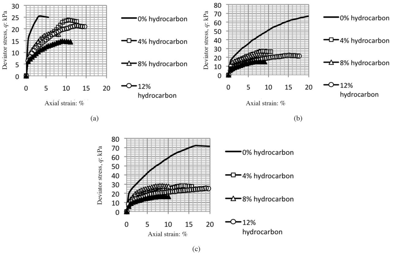
FIGURE 7. The relationship between shear stress and strain for metasedimentary soil with different applied confining pressures of (a) 140 kPa, (b) 280 kPa, and (c) 420 kPa
